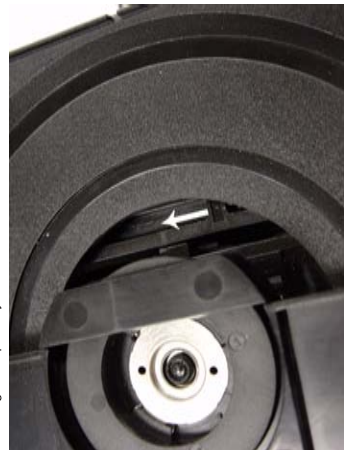
Manually opening of tray When it is not possible to open the tray with the open/close button, the tray can manually be opened. When no disc is loaded, unlock the tray by moving the slide from the left to the right and pull tray outwards.
